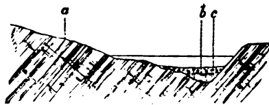
FIG. 80.—Auriferous River-bed; transverse section.
